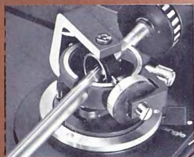
Each gimbal is hand-assembled, and special gauges assure that each will conform to Dual's stringent specifications.
